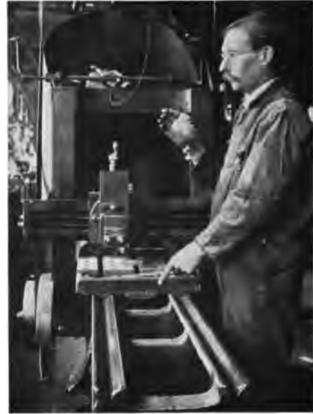
Fig. 2. Man with Hand crushed between Table and Ribs of Planer-Bed.
